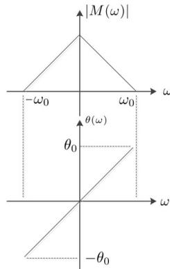
Plot the spectrum of the signal  $\hat{m}(t)$  which is equal to the Hilbert transform of  $m(t)$ .
