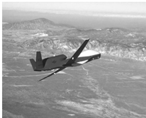
Fig. 1. The Global Hawk Medium Altitude Long Endurance UAV (photo courtesy of US Department of Defense).
