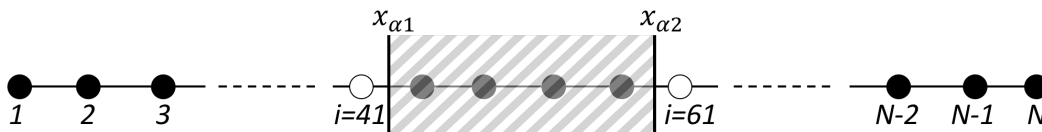
Figure 13. 1D schematic describing the interfaces locations and irregular grid points.
