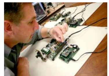
Kevin Carr adjusts the transmitter module that is used to wirelessly link five units being tested in a self-healing computer system.
