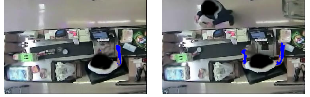
Fig. 2. Hand motion maps detected by our approach. Blue pixels are labeled as hand pixels by the classifier. ( Best viewed in color )
