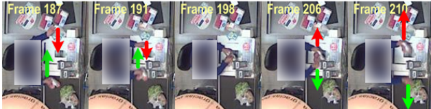
Figure 2. A frequently occurring case in retail: the two hands with identical appearances meet and split in reverse directions. Avoiding identity switching in these cases is a key challenge for tracking both hands.
