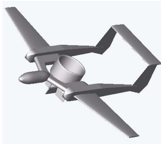
Figure 2. Computer generated representation of the Vertical Take-Off and Landing (VTOL) vehicle currently under development for missions 3 and 4 of the IARC.
