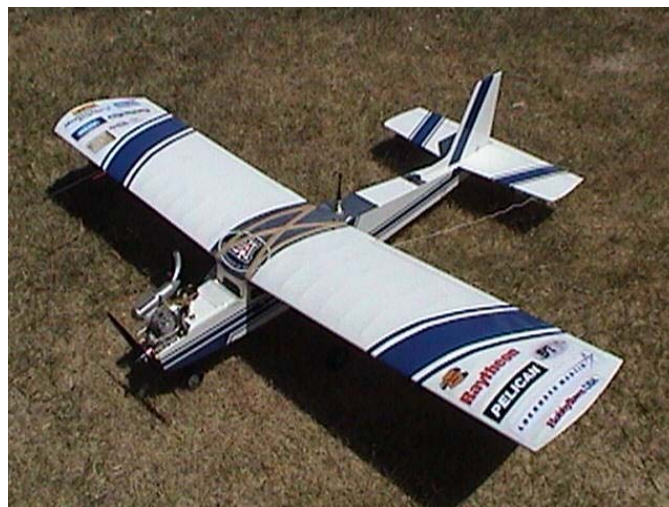
Figure 1. Eagle2 fixed wing vehicle used for 3km, GPS waypoint navigation as well as the target identification and portal detection mission.
