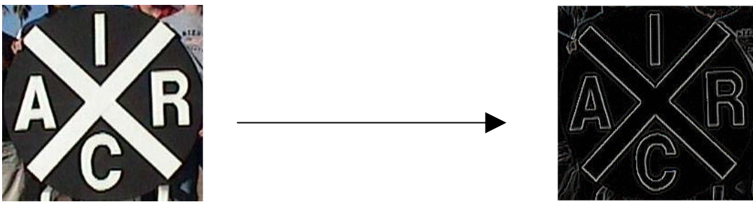
Figure 6. An example of the template at one scale, orientation and viewing angle and its corresponding edge map obtained using the homogeneity operator
