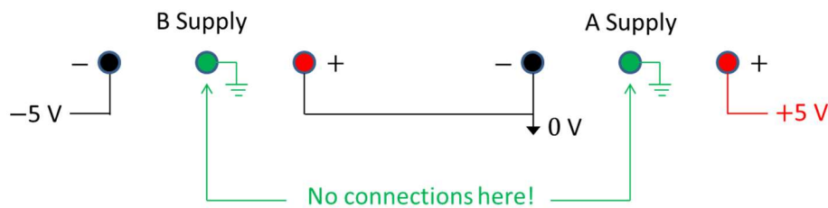
Figure 7. Power supply connections.
