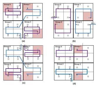
Fig. 2. The layout of different waveguides for (a) layer 0 communication, (b) layer 1 communication, (c) layer 2 communication, and (d) layer 3 communication.
