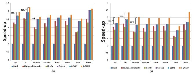
Fig. 5. Simulation speedup for 64-core using SPLASH-2 traffic traces with (a) 64 and (b) 16 wavelengths.
