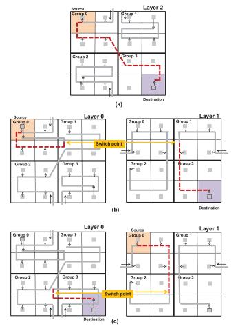
Fig. 4. (a) Static communication between the source in Group 0 and destination in Group 3. (b) Illustration of reconfiguration between Groups 0 and 3 using partial waveguides from layers 0 and 1, and (c) alternate reconfiguration between Groups 0 and 3 using partial waveguides from layers 1 and 0.
