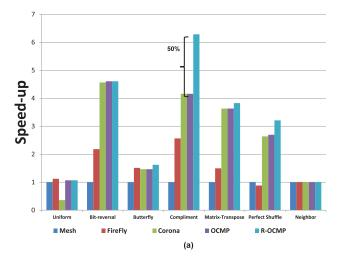
Fig. 7. Simulation results showing normalized saturation throughput for seven traffic patterns for 256 cores.
