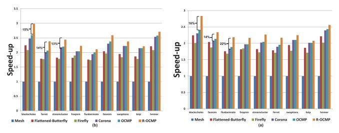
Fig. 6. Simulation speedup for 64-core using PARSEC traffic traces with (a) 64 and (b) 16 wavelengths.
