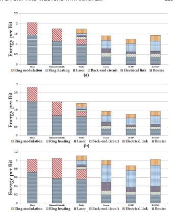
Fig. 8. Average energy per-bit for electrical and NIs: (a) uniform traffic, (b) complement traffic, and (c) butterfly traffic.
