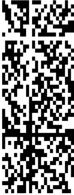
Fig. 6. Shuffled, row-doubled, stacked order-24 Hadamard without dead rows (3456 \mu\text{m} tall, 1296 \mu\text{m} wide).
