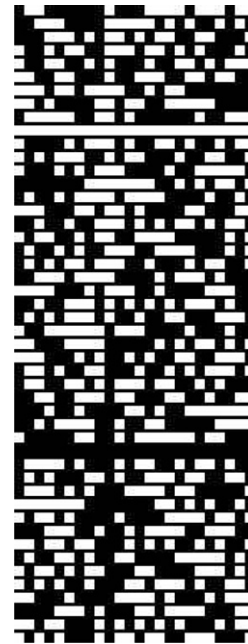
Fig. 5. Shuffled, row-doubled, stacked order-24 Hadamard with dead rows (3456 \mu\text{m} tall, 1296 \mu\text{m} wide).
