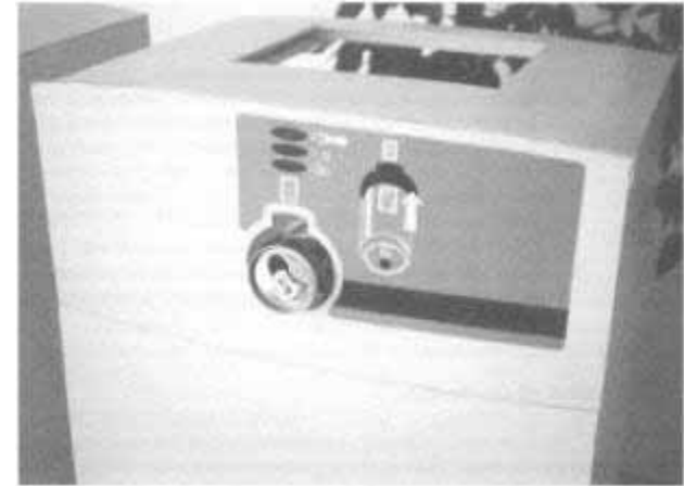
Figure 4.19 The mock-up of the manual version of the can recycling machine. In testing, a visible researcher stood behind the machine to accept or reject each can while another used color pieces of paper to simulate the indicator lights.
