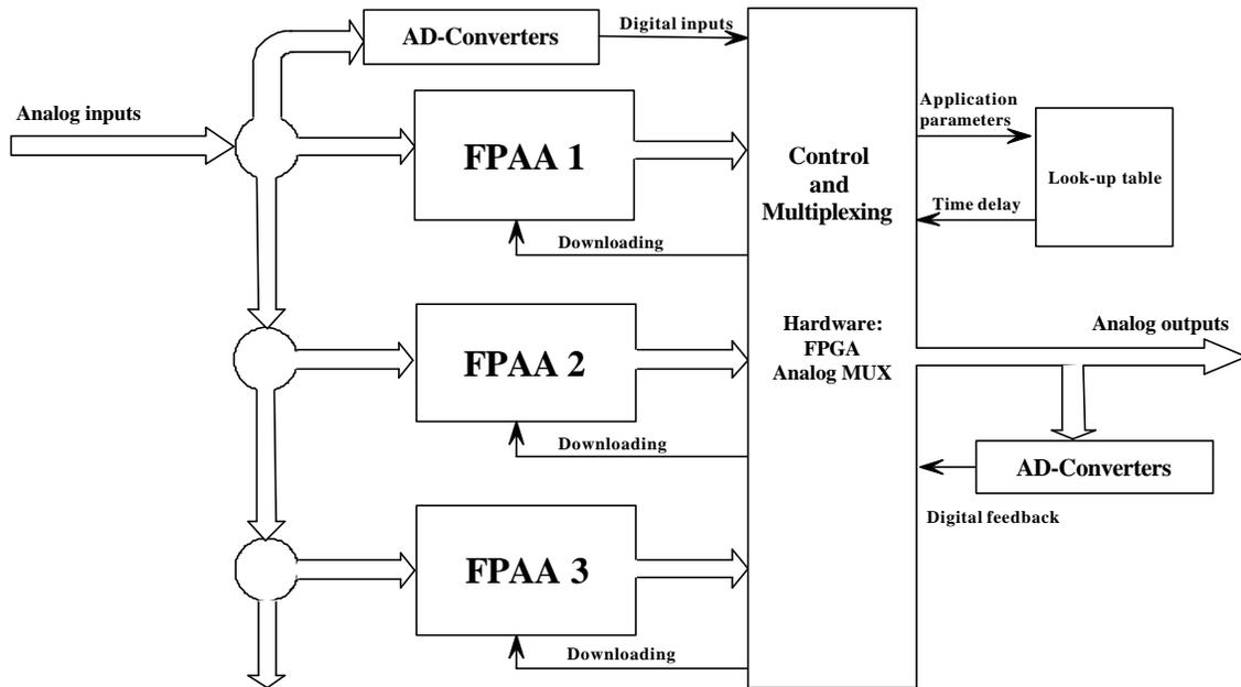
**Figure 10. Block diagram of the system using a FPGA with a look-up table and blocks of programmable chips.**
