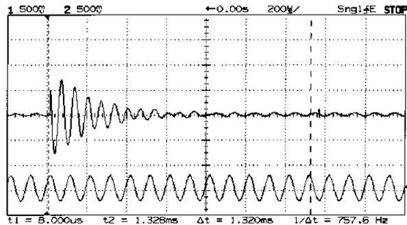
**Figure 3. Settling behavior of band pass filter after switching.**
