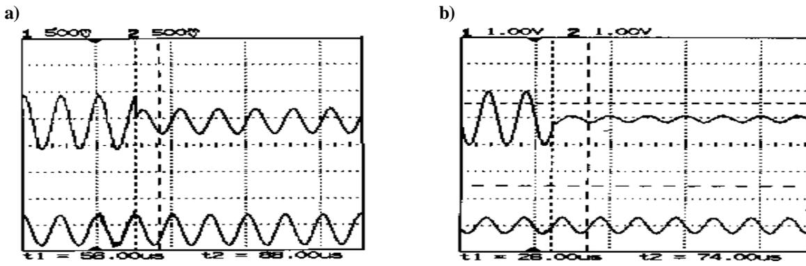
**Figure 4. Switching at zero-crossing after time delay; a) switching near the peak, b) switching close to the zero-crossing.**
