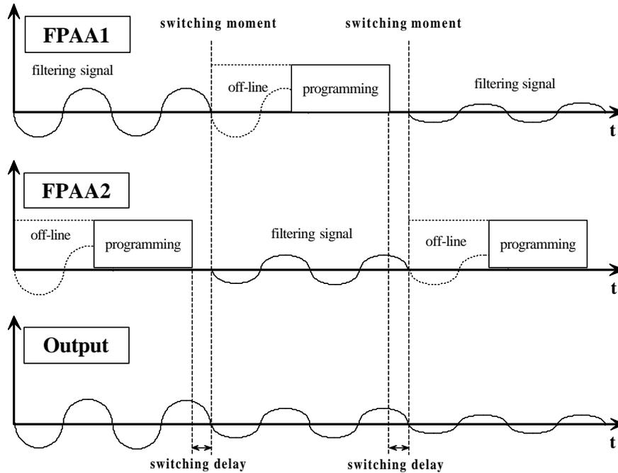
**Figure 2. Timing diagram of reprogramming and filtering of 2 parallel FPAAs for uninterrupted processing of an analog input signal.**
