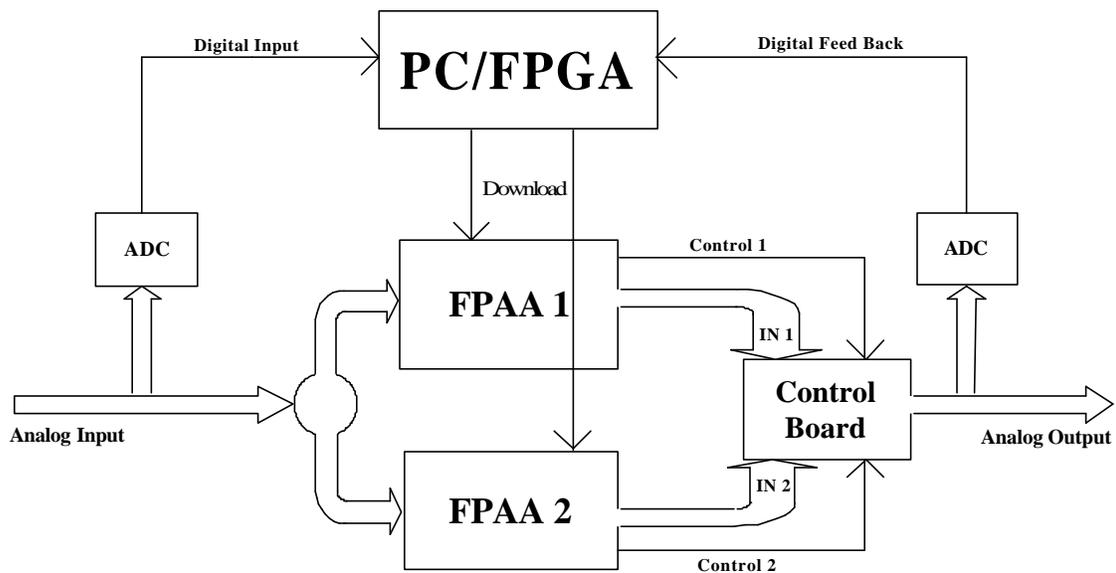
**Figure 1. Block diagram of the system composed of 2 parallel FPAAs.**
