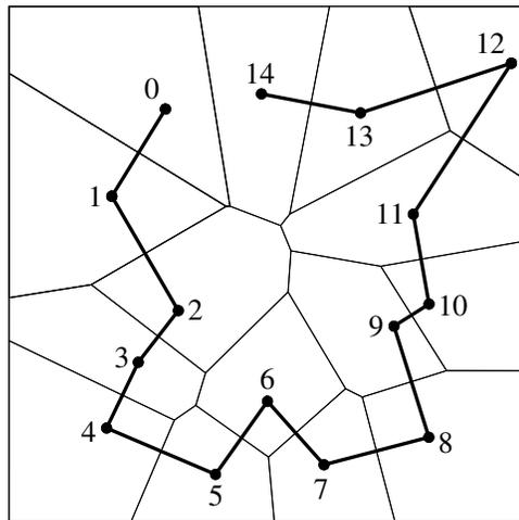
**Figure 1: Voronoi diagram of a 15-node topology where two nodes sharing a Voronoi cell edge (Delaunay neighbors) are 14 hops apart.**
