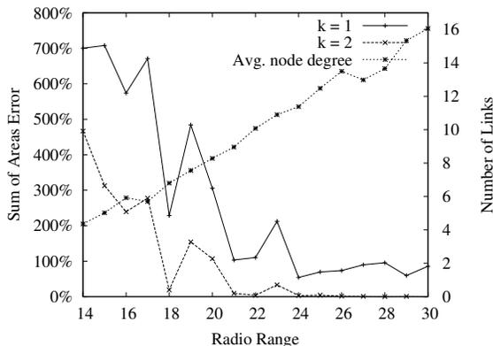
**Figure 2: Relationship between the overestimate of the sum of areas of Voronoi cells and network connectivity. Neither 1-hop nor 2-hop neighbors provide enough information to obtain accurate Voronoi cells in sparse topologies, and computation using 1-hop neighbors under-performs the use of 2-hop neighbors on all tested topologies.**
