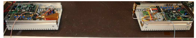
Fig. 16. Transmitter and receiver setup for the BERT measurements. The transmitters were placed less than 1 m apart for this test.
