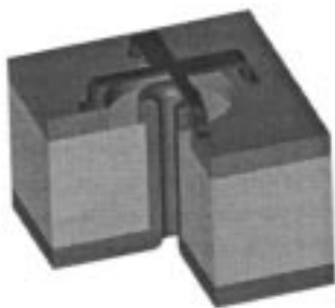
Fig. 6. Improved switch element, off state.
